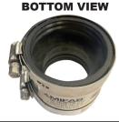
If the 2" PVC socket outlet body with membrane flange is not used, MIFAB recommends the MIFAB # MI-HUB-TR-215 transition no hub coupling to connect the 2" (51mm) spigot outlet to the 2" PVC / C.I. drain pipe. This coupling is not included and is an additional cost.
